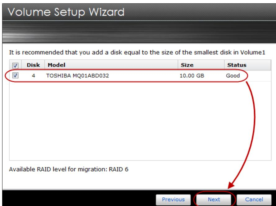
The screenshot shows the 'Volume Setup Wizard' window. The title bar reads 'Volume Setup Wizard'. The main content area displays the text: 'It is recommended that you add a disk equal to the size of the smallest disk in Volume1'. Below this is a table with the following columns: 'Disk', 'Model', 'Size', and 'Status'. The table contains one row with a checked checkbox in the 'Disk' column.
